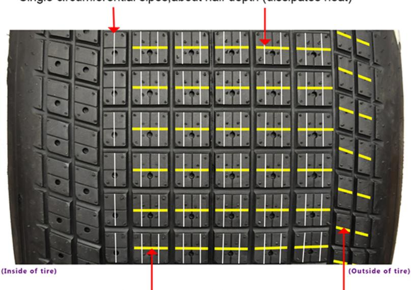
Very narrow groove, approximately 3/4 depth of block Straight across or at a slight angle
